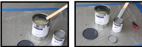
B.) Pour the contents from Part "A" into the larger Part "B" container. Do not mix Glaze Coat with Epoxy. Be certain to empty all the materials from the Part "A" container. Vigorously mix the two components together for at least three minutes. Be sure to scrape the sides and bottom of the containers to assure that all material is properly mixed. Improperly mixed resins may leave soft spots or may cause color variation when applied.
