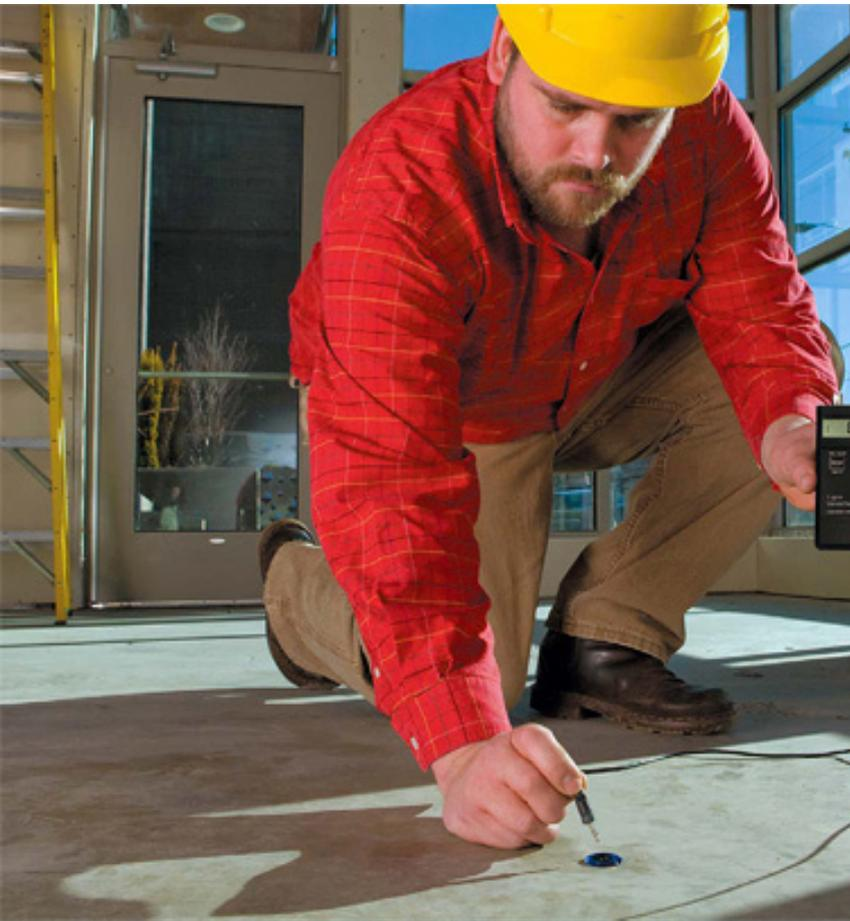
Every concrete slab has a unique profile based on its formula, sub-soil, placement, finish and cure. Concrete moisture testing provides guidance on whether moisture mitigation is necessary.
